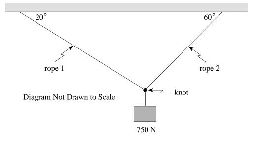
a) Draw a free-body diagram showing the forces acting on the knot. (2 marks)
