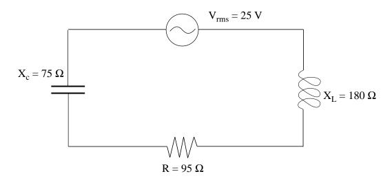
a) If the coil has an inductance of 35.0 mH, what is the applied frequency? (2 marks)
