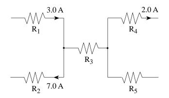
What are the magnitude and direction of the current passing through resistor  $R_5$ ?
