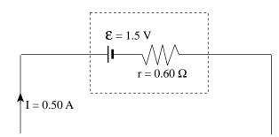
What is the terminal voltage of the cell while being charged?
