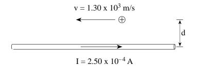
If the magnetic force on the proton is  $1.64 \times 10^{-26}$  N, at what distance **d** is the proton travelling above the wire? (7 marks)
