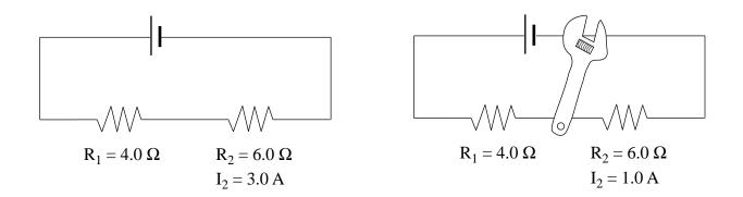
When a wrench that has a small resistance is dropped on the circuit as shown, the current through  $R_2$  is reduced to 1.0 A. What is the current flowing through the wrench? (Assume the supply voltage remains constant.)
