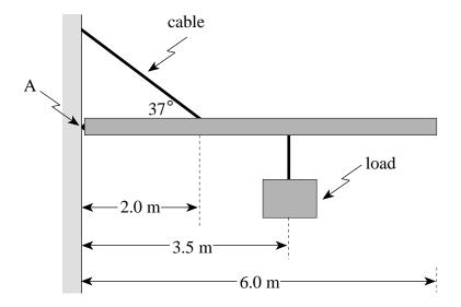
If the maximum tension the cable can withstand is  $2.4 \times 10^3$  N, what is the maximum mass of the load? (7 marks)
