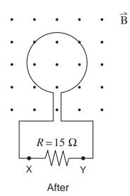
What are the magnitude and direction of the current through the  $15 \Omega$  resistor?
