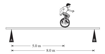
a) When he is at the position shown, determine the forces exerted by the supports on the beam. (5 marks)
