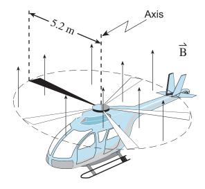
What is the magnetic flux swept out by the rotor blades in one revolution and what is the emf induced between the axis and tip of a rotor blade?
