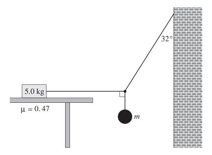
A coefficient of friction of 0.47 exists between the 5.0 kg block and the table. What is the maximum mass, m, that can be hung from the cords before the 5.0 kg block begins to move? (7 marks)
